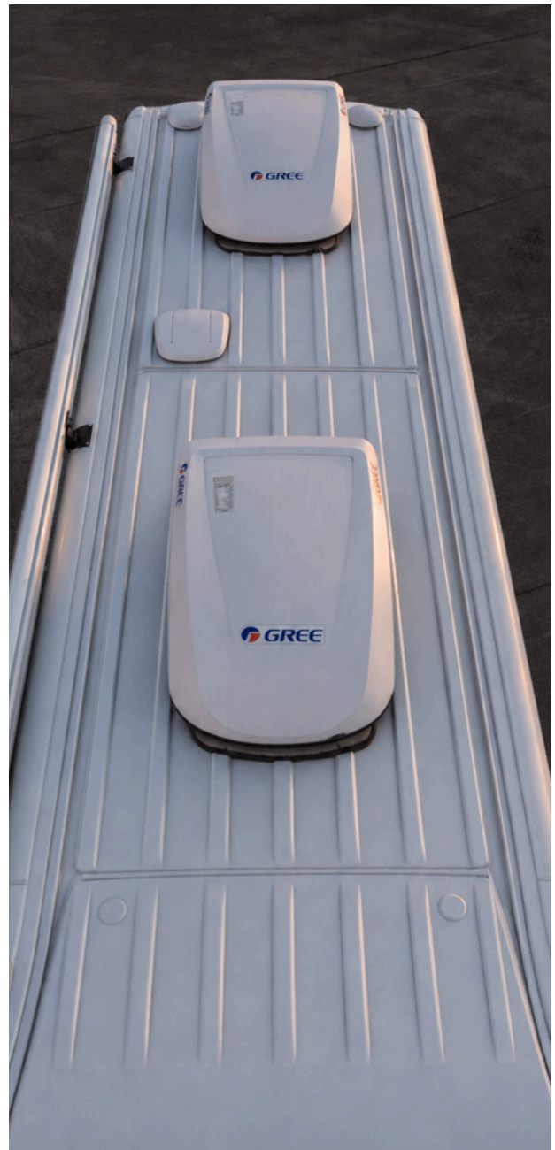
Dual rooftop air conditioning
